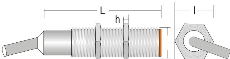
$\emptyset = 18 \text{ mm}$   $L = 76 \text{ mm}$   $I = 28 \text{ mm}$   $h = 4 \text{ mm}$
